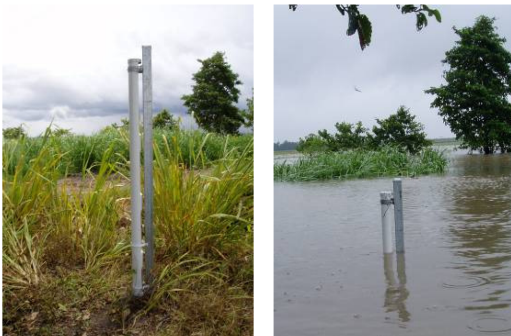
Figure 12 Rising stage sampler located at location 06 before (left) and during flooding.
