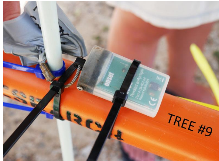
Figure 10: Hobo data logger attached to coral nursery tree
