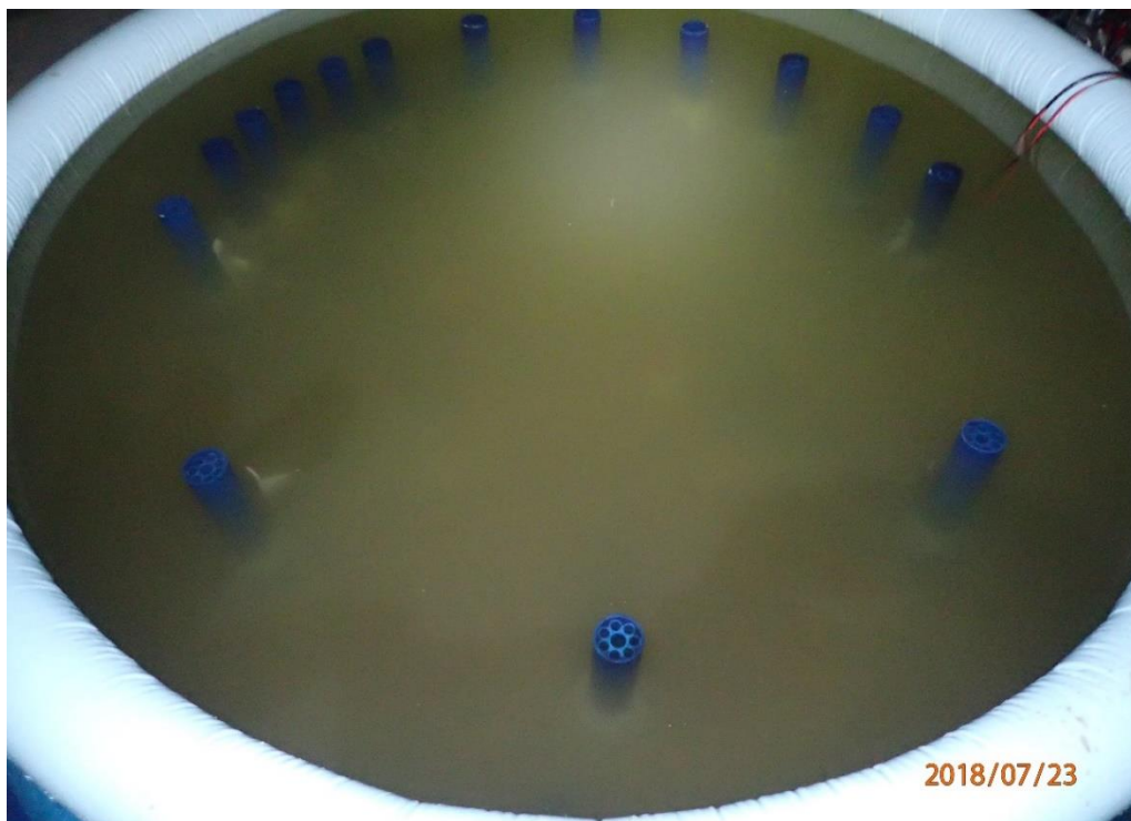
Figure 2.20. Circular flume experiment with 3 replicate traps and a head and tail trap at each 0.65D, 3D and 9D spacing.
