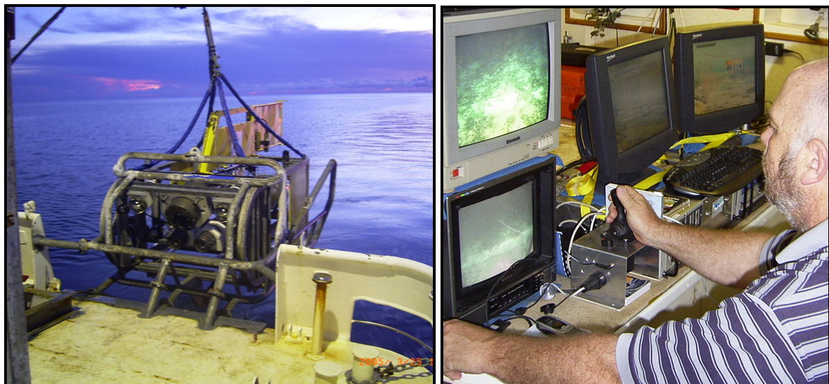
Figure 2. The Drop-Cam system recovered after completion of a 500 m video transect and the surface real-time monitoring, control and data acquisition system.
