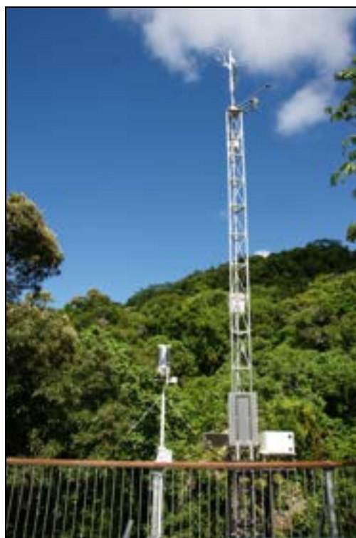
Figure 1: Eddy covariance (EC) and weather station instrumentation on the Discovery Tower.
