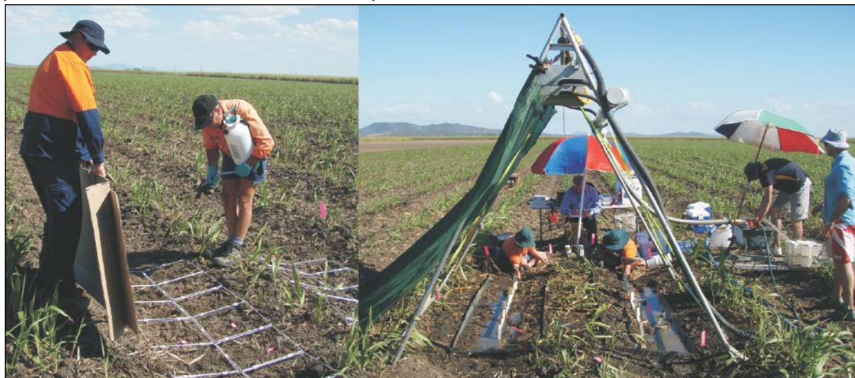
Figure 1. Rainfall simulation trials were carried out in the Burdekin and Mackay Whitsunday regions to examine the runoff of the key and emerging products used in the sugarcane industry.
