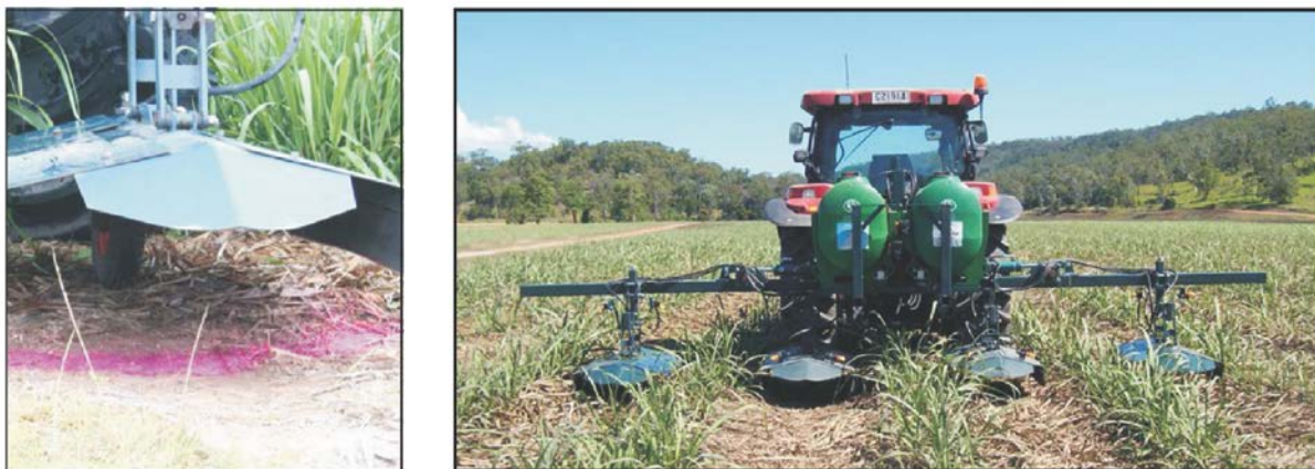
Figure 8. The WeedSeeker technology has been applied in the Mackay Whitsunday region and can reduce application of some herbicides by up to 80% (from http://reefcatchments.com.au/files/2013/02/WeedSeekerSm1.pdf ).
