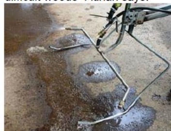
The spray bar showing centre air induction nozzle for glyphosate
