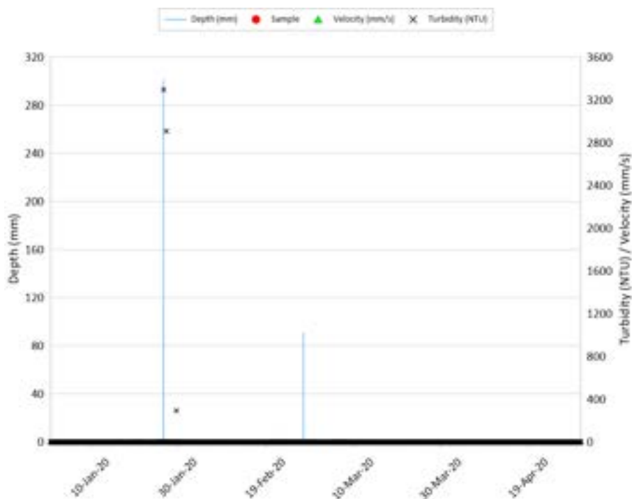
Figure 87: Virginia Park Control gully runoff, turbidity, velocity and sample points on the hydrograph. Event threshold = 300 mm.
