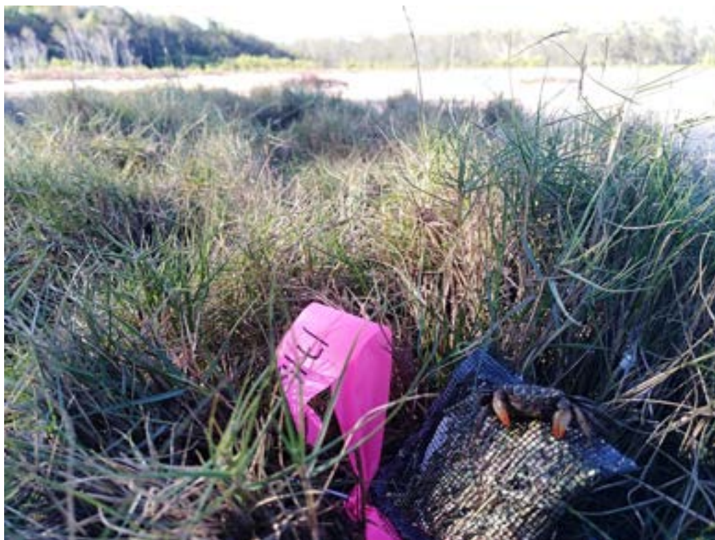
Figure 6. Example of surface deployed decomposition bag at a high marsh site. The bag was tethered to an aluminum spike in wetland.
