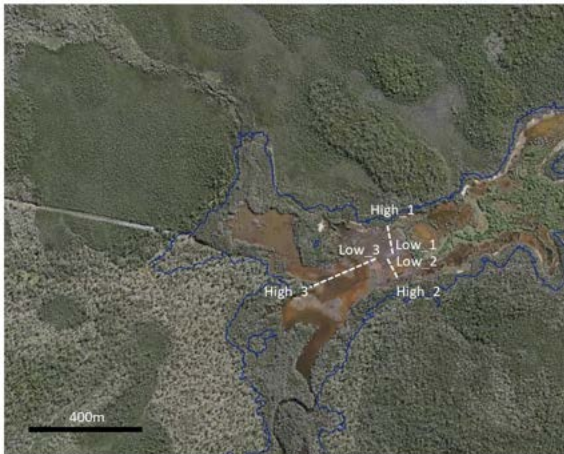
Figure 5. Example transect design for the Round Hill Reserve survey location. Three low elevation survey points were placed at the start of the mangrove tree line, and corresponding high elevation survey points were placed at the start of the terrestrial tree line. Five replicates at each survey point were spaced ~2-3 meters apart and in parallel with the tree line. Blue line is the Highest Astronomical Tide level (Queensland Government Globe spatial data).
