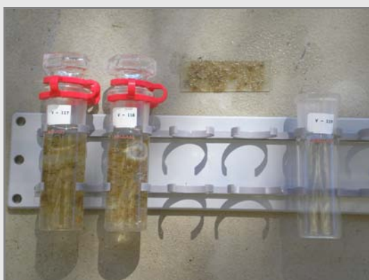
Figure 7: Custom made glass vials for net oxygen production and respiration measurement of biofilms.
