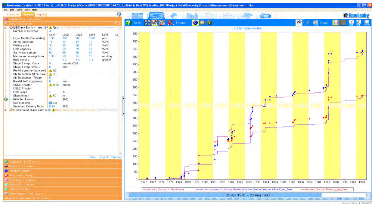
Figure 9: Simulated and measured cumulative runoff and soil erosion from the stubble burnt –winter crop catchments at Greenmount (1976-1990)
