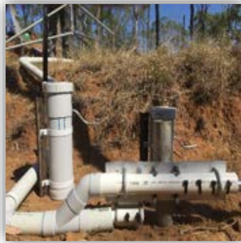
Figure 9: (A) Example of a treatment gully set up and (B) and example of a control gully set up including two rising stage samplers
