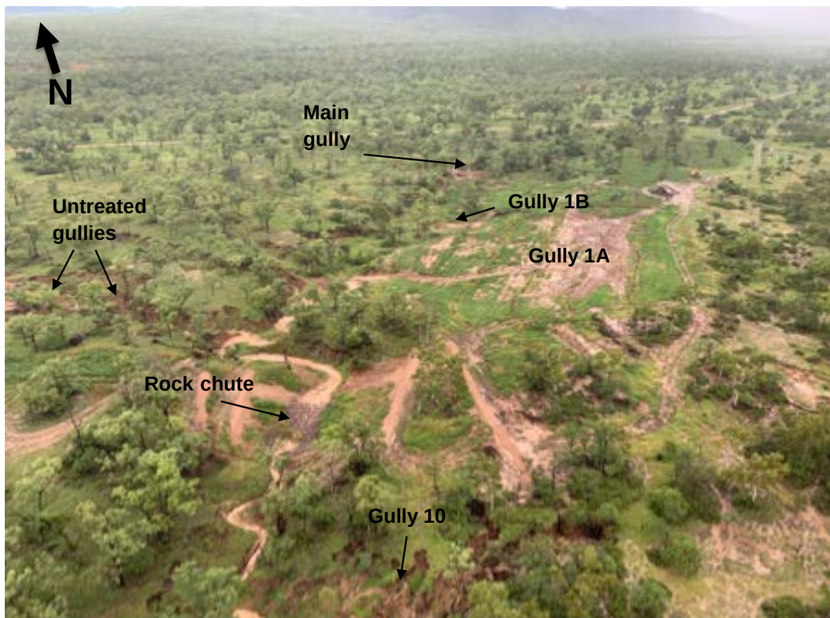
Figure 49: Image taken during sample collection for the January/February rainfall event (Photo credit: Damon Telfer). Note the area under the gully 1A text with little vegetation as a result of works to repair holes and tunnel erosion following the heavy rainfall in July (Source: NQ Dry Tropics)
