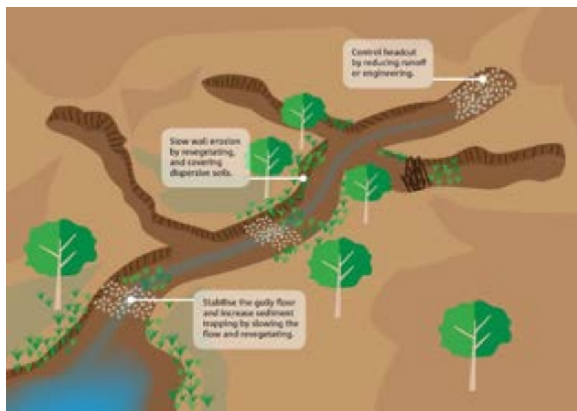
Figure 2: Conceptual model of the outcome of various treatment options within a gully (Wilkinson et al., 2019).
