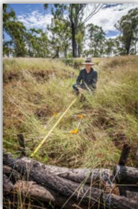
Figure 38: (A) Example of the stick traps installed at MinnieVale station and (B) measurements of the vegetation cover and biomass behind the stick straps at this site in April 2019.
