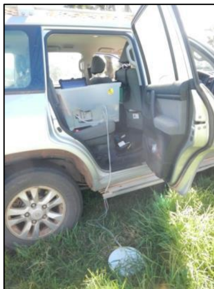
Figure 13: Measurement of gaseous emissions using the INNOVA gas analyser (in vehicle) and closed chamber.
