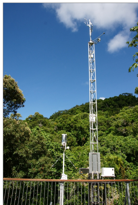
Figure A3: The Discovery Tower eddy covariance system.
