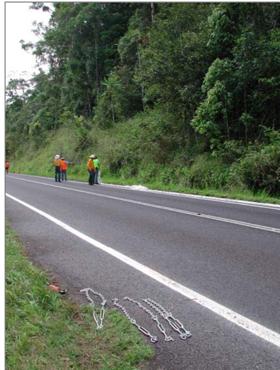
Figure 2.11 Turnbuckles and chains for attachment to pole and wooden supports on trees. Photos courtesy of Nigel Weston.
