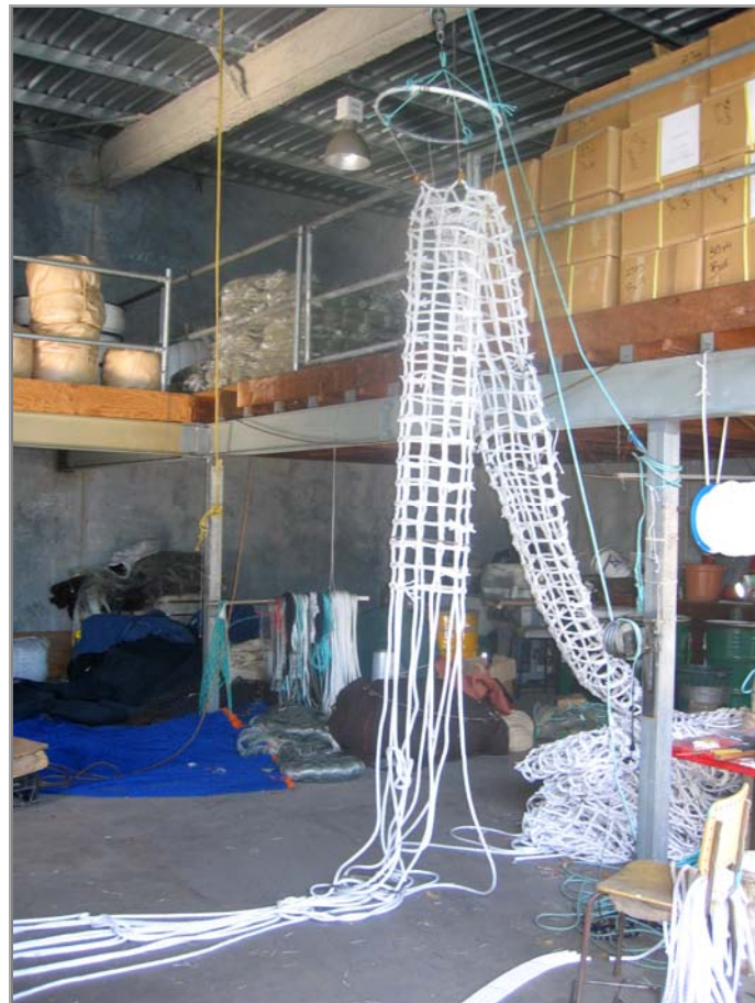
Figure 2.7 Rope tunnel under construction at Gulf Net Menders Pty Ltd. Photo courtesy of Nigel Weston.
