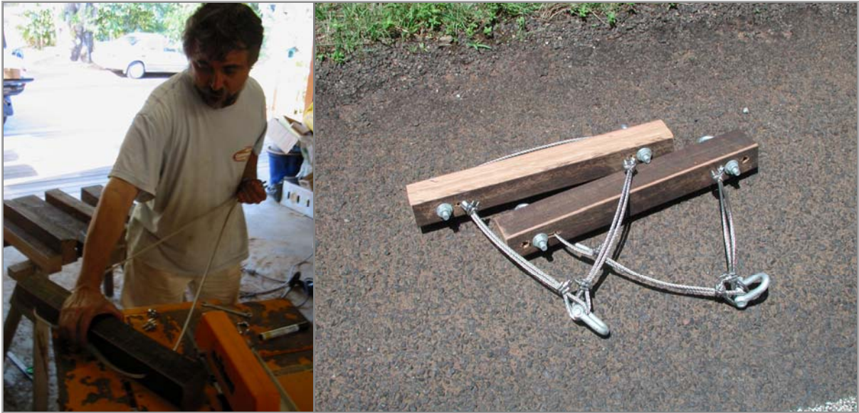
Figure 2.6 Wooden supports used in attaching the canopy bridges to tree trunks, ( left ) created in the home workshop, and ( right ) the final product. Photos courtesy of Nigel Weston.
