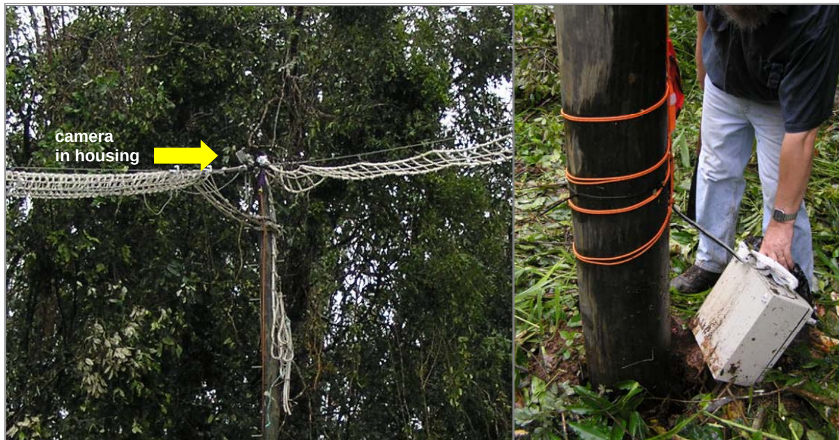
Figure 3.2 (Left) Inconspicuous camera in position facing along the rope tunnel, and (right) the control box for downloading images and battery with cable leading down from camera. Photos courtesy of Steve Goosem and Miriam Goosem.
