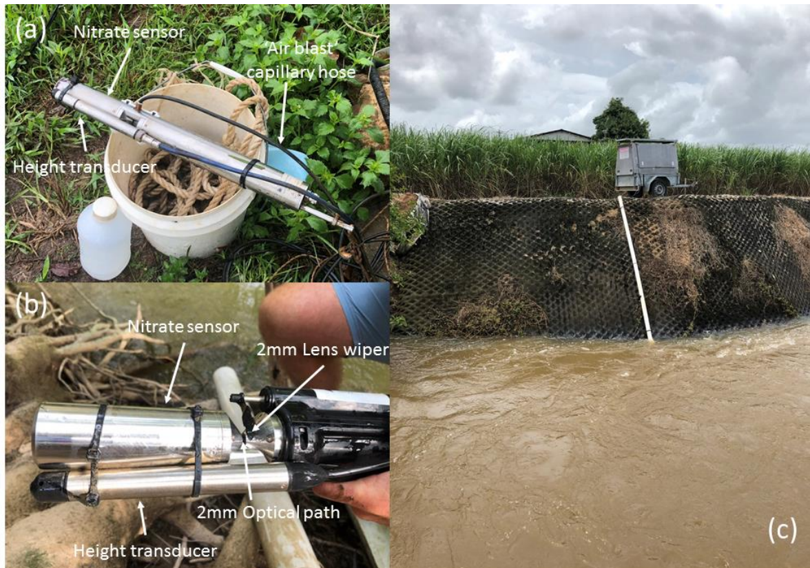
Figure 3: Alternative optical lens cleaning options utilised throughout Project 25. (a). Compressed air blast; (b) Automated, externally mounted lens wiper currently being trialled. (c). Real-time monitoring station during wet season flood event.
