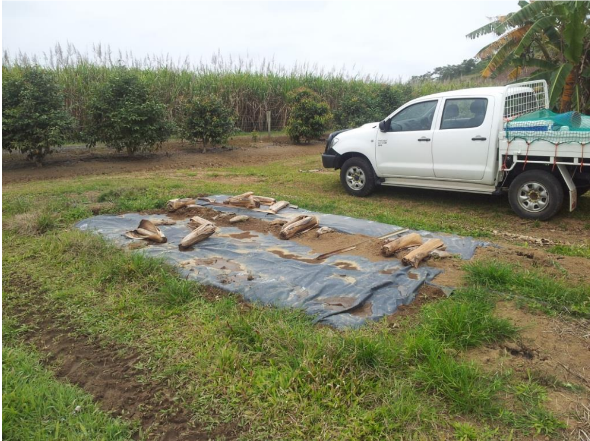
Figure 9 An area of soil was covered with plastic to prevent evaporation and ‘wet up’ for the purpose of determining the upper water holding capacity of the soil.
