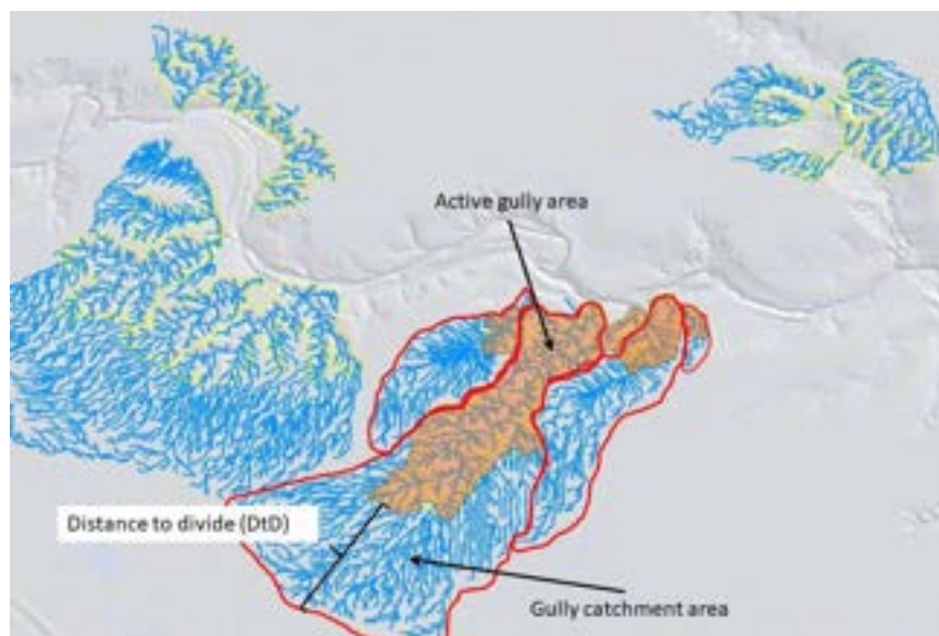
Figure 37: Schematic diagram showing the relationship between active gully area and gully catchment area in an alluvial gully.
