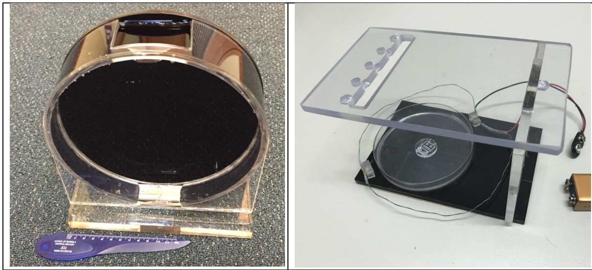
Figure 2: Viewing chambers provided to stakeholders to improve the quality of images submitted for identification by experts. (A) Transparent sides and front provide strong lighting to photograph specimens and the black background enhances the contrast of specimens. (B) Low-cost perspex design in which a petri dish is mounted between LEDs (powered by a 9v battery). A smartphone rests on the upper perspex sheet (focusing through the large slit), which also contains magnification lenses (the smaller holes).
