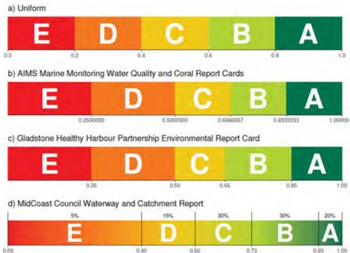
Figure 77: Score to grade conversions. In each case, the scale along the base defines the grade boundaries.
