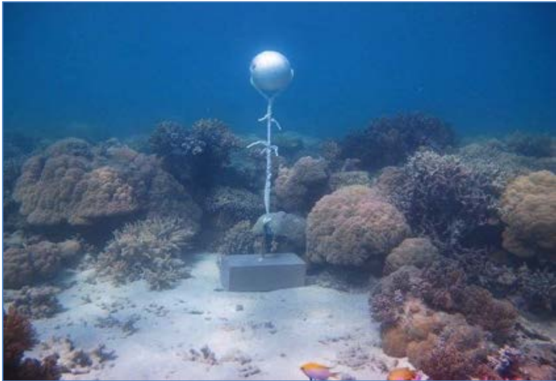
Figure 4-15: Temperature logger deployed on a small concrete block with a float for visibility.
