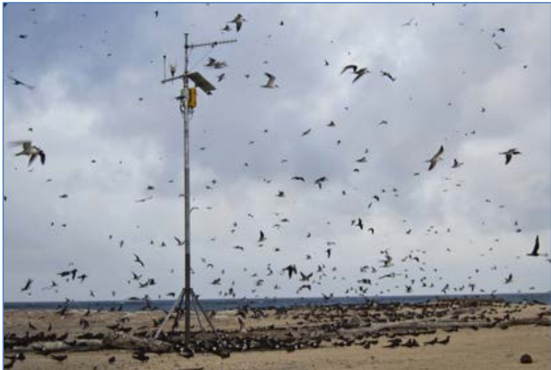
Figure 4-16: Land based component of the Bramble Cay weather station.
