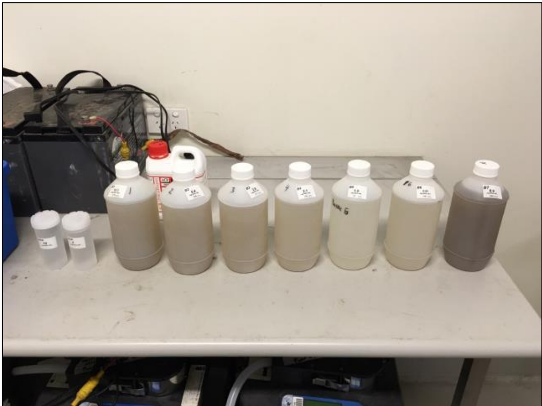
Figure A1: Laboratory testing of SUNA with various nitrate-suspended sediment samples to test performance against potential field conditions.
