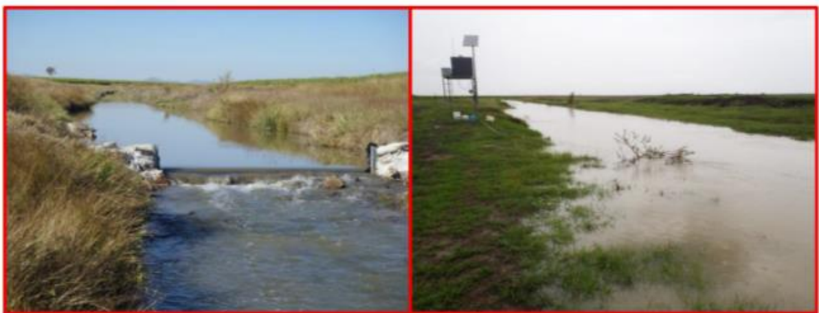
Figure 27: A typical irrigation event (left) and typical flood event from major rainfall (right) flowing past the monitoring station instream control feature (the elevated RTWQM station platform is visible in right picture).
