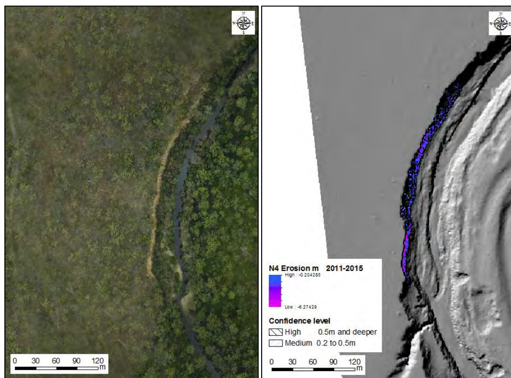
Figure A38: The largest patch of erosion that was not bedload was from this 11m tall bank on the East Normanby main channel, with a volume of 23,754\text{m}^3 .
