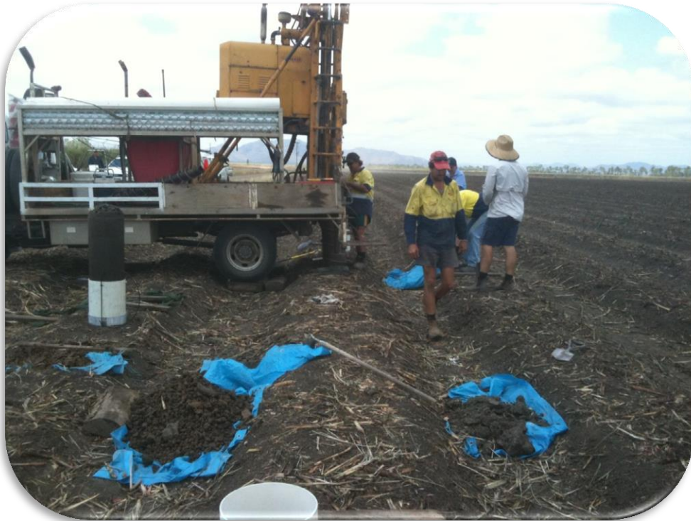
Figure 5. Preparation for installation of lysimeters in the ground with specialized coring equipment that collects the intact cores, on which the lysimeter base and ring is placed before the placing the lysimeter and core back into the ground.
