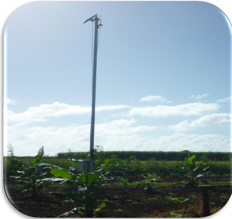
Figure 11. MEA Magpie sensors for continuous monitoring of change in soil moisture, temperature and electrical conductivity to 120 cm depths in the micro-sprinkler irrigation block.
