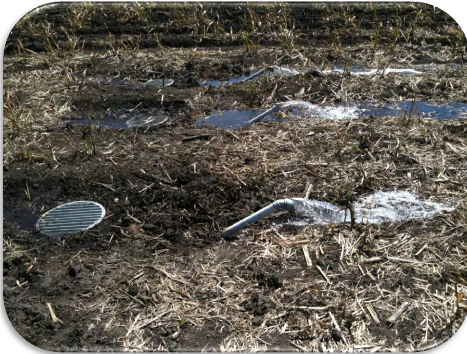
Figure 1. Installation of pit trap for monitoring of surface flow and sample collections from sugarcane paddock.
