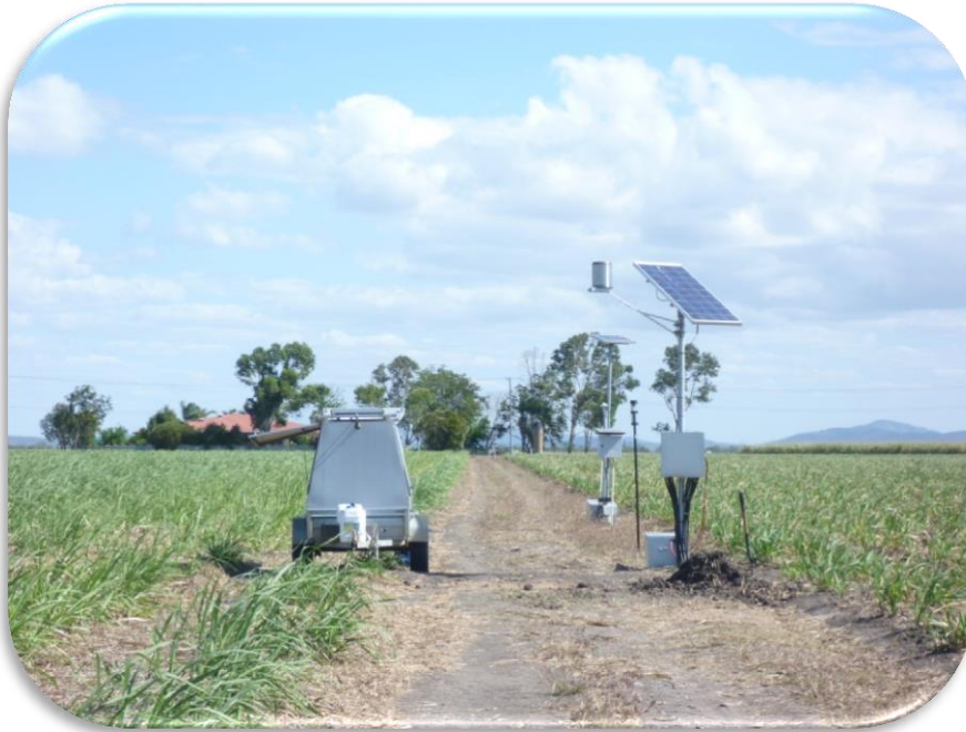
Figure 3. Instrumentation for rainfall and irrigation water input monitoring, measurements and sampling of run-off (over land flow), and deep drainage from the furrow and SDI block in the sugarcane trial at Home Hill, Burdekin.
