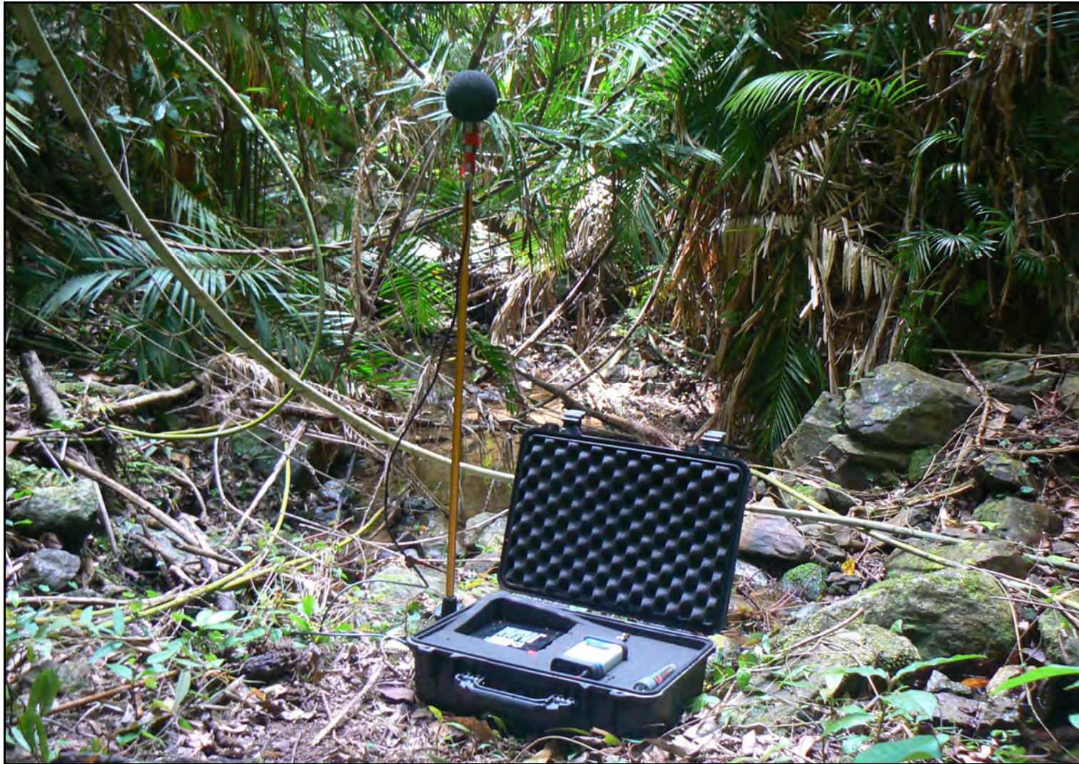
Figure 1: Sound level meter setup at upper Streets Creek acoustic refuge, 170m from highway along Powerline transect.
