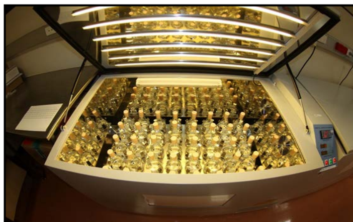
Figure 2: Flask experiment in incubator shakers to test the persistence of herbicides under standard conditions. Image P. Mercurio.
