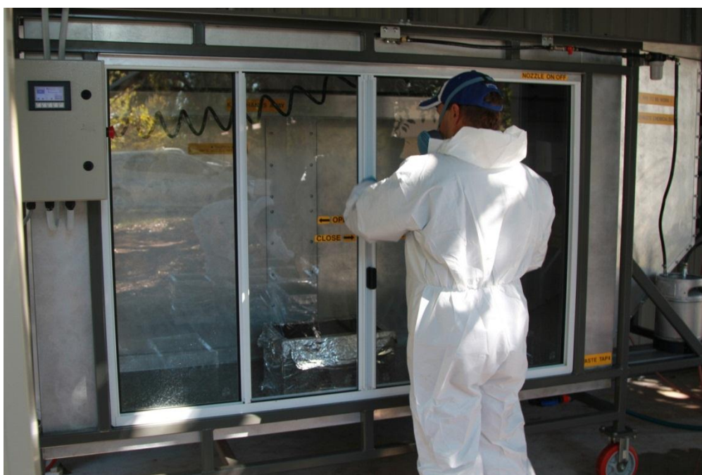
Figure 7. Spray cabinet in which herbicides were applied to soil and crop residue
