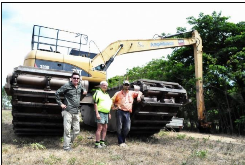
Figure 17: Civil Plus Construction's amphibious excavator with Greening Australia staff (left), property owner (centre), and excavator operator (right). This floating excavator completed the works in just seven days, progressively moving along the creek, picking up the floating invasive weeds and relocating to the banks for drying and later used for mulching on nearby tree planting (Photo source: Greening Australia).
