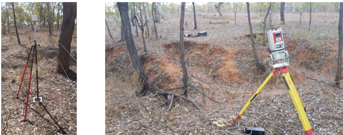
Figure 4: (left) a survey bipod with cylindrical reflector and (right) the RIEGL TLS at the gully site
