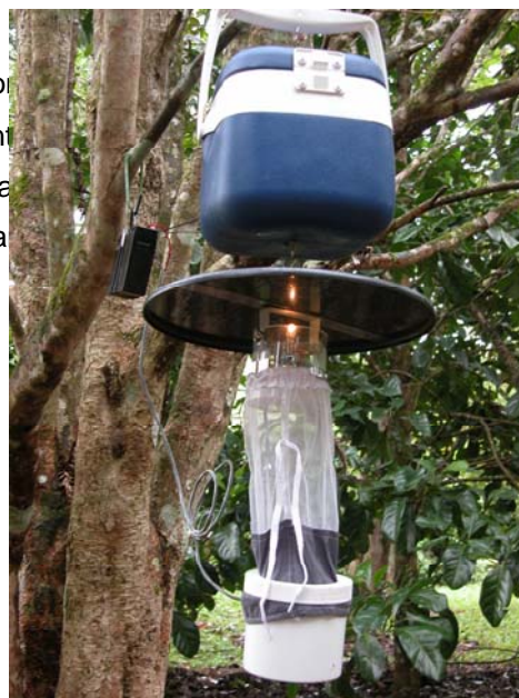
Plate 1. Our implementation of the international standard "CDC", US Center for Disease Control mosquito trap with a small light and an insulated container of dry ice producing CO 2 as attractant.
